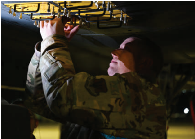
▲ An Air Force airman installs a countermeasure firing pulse tester into a U.S. Air Force F-15E Strike Eagle at RAF Lakenheath, England, last May to assess EW defensive system readiness. Air Force photo
