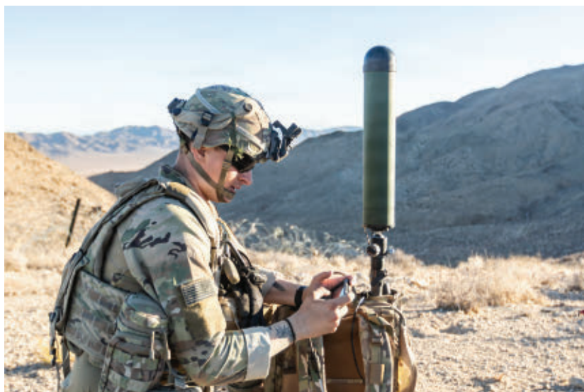
▲ An Army electronic warfare specialist uses a Mastodon Beast+ system at an exercise last month. Mastodon Beast+ system is a multi-channel electronic warfare device designed for detection, direction finding, and attack of adversary signals. Army photo
